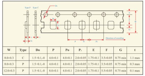
NOTE : The nominal Dimensions of the component compartment (A<sub>0</sub>, B<sub>0</sub>, K<sub>1</sub>) are derived from the component size. C = PAPER P = PLASTIC
